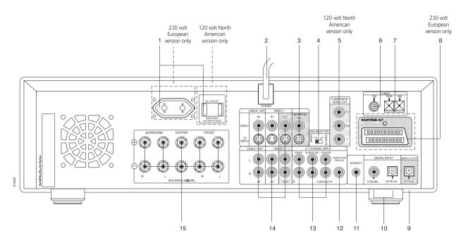
SWITCHED AC OUTLET: This convenience jack can supply switched power to another component or accessory. It is powered on and off by the front panel POWER key (or the HTR L70's ON and OFF keys).
